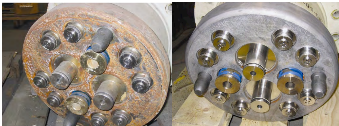
Corroded part of oil platform equipment
