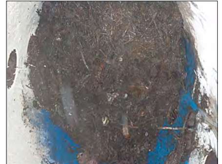
Close-up of digestate after the 28 days. White specs in the photo identified as mold.
