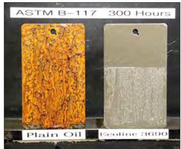
This ASTM B-117 salt spray test shows that a coating of EcoLine® 3690 protects metals for 300 hours in 100% humidity with no rust. Further tests have shown the same results with over 2,000 hours logged.
