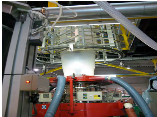
Ecocortec's High Tech Blown Film Extrusion Line for Biofilms in Beli Manastir, Croatia
