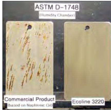
EcoLine® 3220 provides long lasting vapor corrosion inhibition and is made from renewable materials. Here is EcoLine® 3220 tested in comparison to another commercial product.
