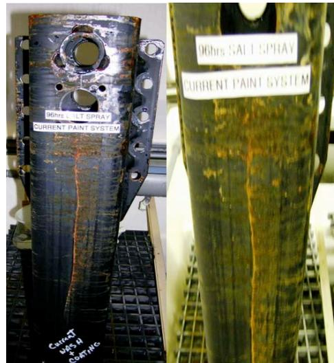
This pole had the current paint system. The pole was scribed and placed in the salt spray cabinet for testing.
