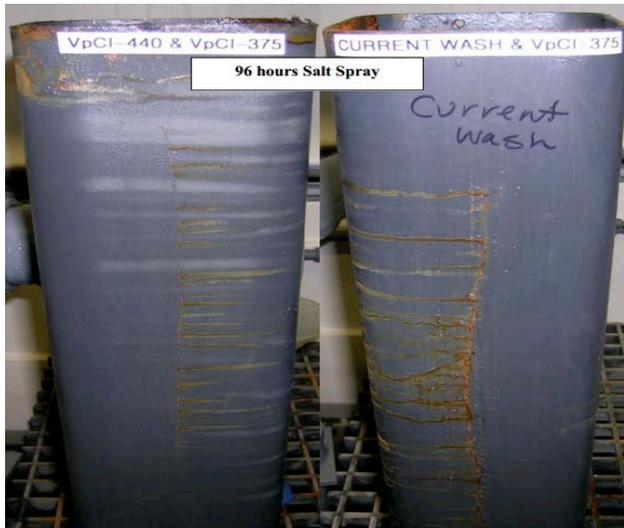
VpCI®-440 was scrubbed onto the pole and allowed to dry for 1 hour. VpCI®-375 was sprayed onto the poles at 6 wet mils and the poles were left to dry for 7 days. The poles were scribed and placed in the salt spray cabinet for testing.
