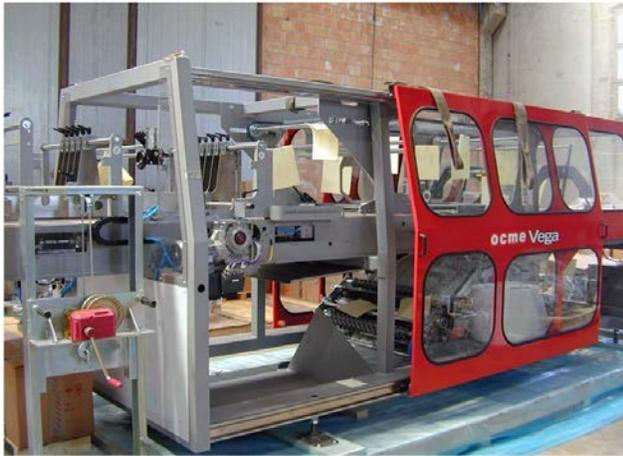
**In transport corrosion protection using Cortec's VpCI<sup>®</sup> 132 foam of shrink-wrapping machine for PET bottles.**
