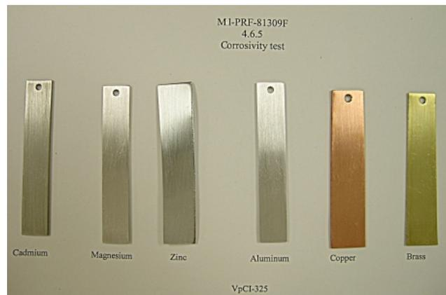
**Specimens that were immersed in VpCI-325, after 1 week. All specimens display no corrosion.**
